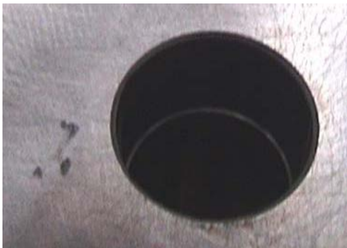
Fig.2 damage on the surface due to metal locating pin
