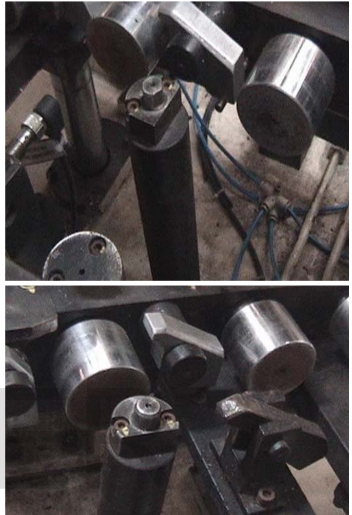
Fig. 3 metal locating pins
