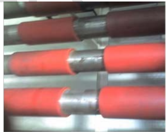
FIG .1 METALLIC ROLLERS WITHOUT & WITH RUBBER COATING
